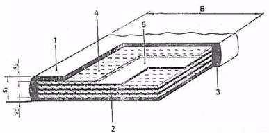
Fig. 1. Parts of textile insertion conveyor belts: 1-carrying rubber face; 2-rolling rubber face; 3-rubber edge; 4-insertion; 5-intermediate rubber (linking inserts);  $S_1$ -belt thickness;  $S_2$ -supporting face of the belt thickness;  $S_3$ -rolling face belt thickness; B-belt width;
