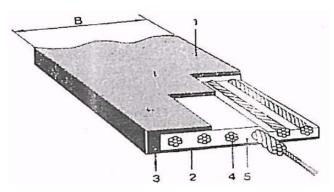
**Fig. 2.** The structure of transport belt with steel cable insertion: 1-carrying rubber face; 2-rolling rubber face; 3-rubber edge; 4-steel cables; 5-rubber layer linking cables; B-belt width;
